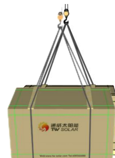
Figure 6 Schematic diagram of Module lifting
